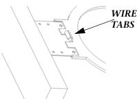
Step 4: After the wall board is installed, cut out the hole for the speaker using the inside cut-out of the frame as a guide. The
