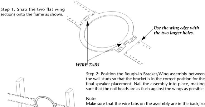
Make sure that the wire tabs on the assembly are in the back, so they are on the inside of the wall.
